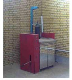
This device use for shock test of porcelain insulators before electromechanical and puncture test
