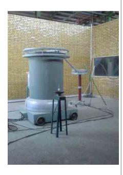
This instrument capable us to use it on test of all products in an electrical routine test also it use in all sample test like wet power frequency test, puncture test and also it providing electrical current in electro mechanical test. This device have calibration certificate and this process will be done periodically.
